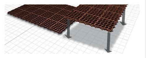
ECORASTER® is simple and quick to install without special tools or equipment. The system is pre-assembled in 3 x 4 pieces (approx 33 x 33 cm) can be efficiently installed in large sections. 14,31 sq ft are installed with a single movement.
